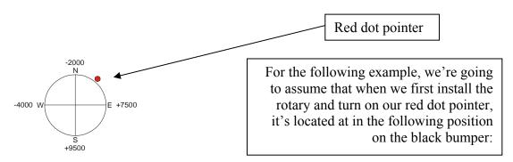
We need to move the red dot a little South (S) and a little East (E). We'll adjust the Y-axis first. We need to move the red dot to the South (towards +9500). Press the Config button, and then the left or right cursor buttons until you get to the Y R Home: menu item. We need to increase this number, but not by much, so we'll press the Up cursor button to increase the number to +0150. Next press Go, and then Reset. The red dot will move to its new Y Home position:
