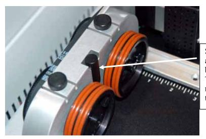
Set your cylinder on the rotary attachment so that it is close to the black bumper, but not touching it. The cylinder may not be able to rotate freely if it is rubbing against the bumper.
