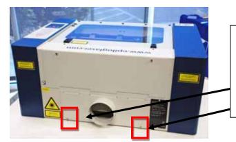
Periodically clean the exhaust plenum at the back of the laser.
