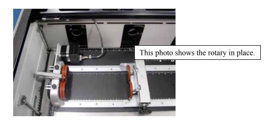
5. Route the connector cable as shown below. This routing prevents the cable from being pinched by the X-Beam when it travels to the back of the machine during the initialization sequence at power-up.
