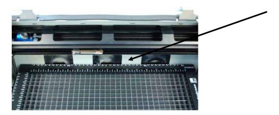
When the vector grid is properly located, you should feel the locating pins click into place. Gently press down on all four corners of the grid to insure it is level. Your vector gird is now installed.
