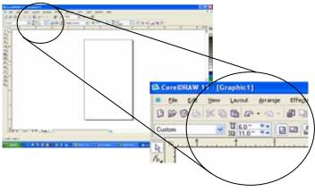
Place your artwork close to the top edge of the page layout. When the job starts, the first part of the process is for the cylinder to rotate through any white space that is between the top of your page and the top of your artwork. Once it has rotated through the white space it will begin to laser your artwork.
