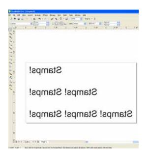
The Fence method uses a *closed outline* to define the area to be engraved away. This image shows the stair-step outline of a Fence enclosing the words to be stamped. The laser will engrave away only the background area outlined by the Fence (leaving the letters standing, of course!).
