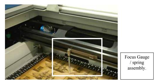
To focus, release the focus spring from its holder on the X-beam. Press the *Focus* button so activate the Up and Down *Arrow Keys* on the control panel. Pressing the Up or Down *Arrow Keys* moves the table. Your machine is in correct focus once the end of the spring just touches your material. Swing the spring back into
