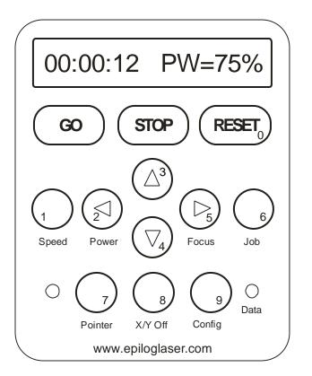
Pressing the **POWER** button while raster engraving will change the display to show the Power setting of the job while it is running (see diagram above). Pressing the **UP** or the **DOWN** key will increase or decrease the power output of the laser in Raster Mode. Normally you will need to increase or decrease the Power by 10% or more before you start to notice a visible change. You cannot change Power on the fly in Vector mode.
