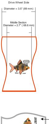
Divide the drive wheel side by the middle diameter and multiply by 100 to calculate the percentage of adjustment. For our example the calculation is:
