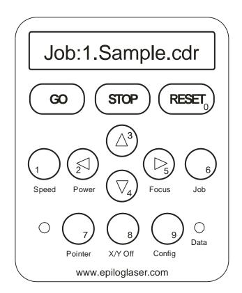
Once the job starts, the display changes to show a job timer and the engraving resolution. The timer is a useful production tool that displays the elapsed time of engraving.
