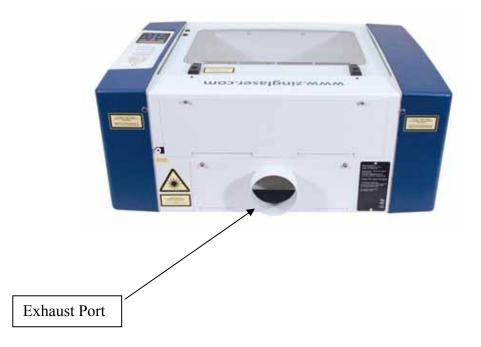
Use flexible aluminum or galvanized sheet metal ducting to connect the laser systems exhaust port to the intake side of your exhaust fan. Then connect the exhaust side of the exhaust fan to the metal duct leading outside.
