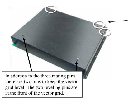
These three mating pins fit into slots that are cut into the rulers
