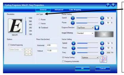
The Job Type: menu allows you to specify Raster, Vector, or Combined. This setting works in conjunction with the way your artwork is setup to produce a raster engraving, a vector profile, or a combination of the two modes in a single job.
