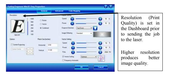
Speed and Power settings are dependent on resolution setting. For example, there is greater overlap of each raster line at 500 DPI than there is at 300 DPI. The additional overlap at 500 DPI has the effect of lasering over more of each line twice. This means that on material like wood, you will notice a greater depth of engraving at 500 DPI than you will at 300 DPI if you use the same Speed and Power settings.
