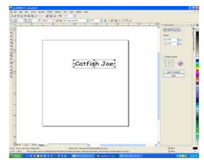
4. Create your artwork so that it is sized to fit into the available engraving area. In this example, we sized the text to fit within the available engraving area. 18 point text fits nicely into our box. Notice that the exact location of where you place the artwork is not important. At this point your artwork is ready.
