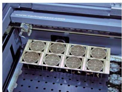
The photo below shows the small pieces from the previous photo laying on the Parts Lifter. Simply lift the Parts Lifter from the Pin Table and throw away the pieces. Cleaning up with the Parts Lifter makes clean up easy because you do not have to
