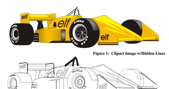
The upper image is a complex piece of clipart. The lower image shows all of the hidden lines that are in this piece of clipart. If this clipart image were run in *Combined mode* it would first raster most of the car then vector cut all but the thickest lines.
