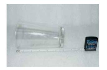
For the width (x-direction) of your page, lay the glass flat and orient it as it will be oriented on the rotary attachment. For this glass, the width of the page will be six inches (152 mm).
