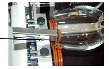
The glass in the photo does not require the use of the clamp. In fact, most standard cylindrical shapes do not need the clamp. The clamp is used mostly for hard to rotate cylinders or very light weight objects that need more than just gravity to hold in place.
