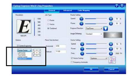
The Center Engraving Option allows you to define the center of your artwork as the primary reference point (Home position) of your engraving or cutting. The Center Engraving Option has been designed to be used in conjunction with the Set Home feature of the laser. This differs from standard printing where the upper left corner of the page and the upper left corner of the laser table define your primary reference point. There are four options for centering your artwork:
