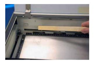
Clean the vents from the inside of the machine. It is best to use a flexible plastic or wire brush that can access the inside of the vent.
