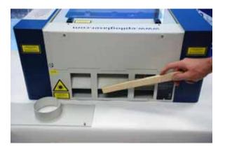
Clean the plenum with a flexible plastic or wire brush that can access the inside of the port.
