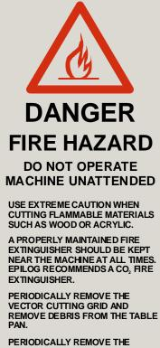
PERIODICALLY REMOVE THE EXHAUST TUBE ADAPTER FROM THE BACK OF THE MACHINE AND REMOVE ANY DEBRIS FROM THE EXHAUST PORT.
